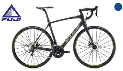
Built to keep you rolling smooth and fast on those all-day rides no matter what the road conditions are. Climbing OR bombing down descends! Equipped with Shimano 105 (2x11) drive-train and TRP's mechanical disc brakes. 2.8" tyres for comfort and performance and still weighing at under 9kg.
